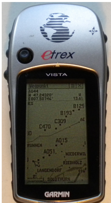
Figure 6.3: Thermal hotspots imported as waypoints on a Garmin eTrex Vista©. Hotspots are marked here as big dots.
