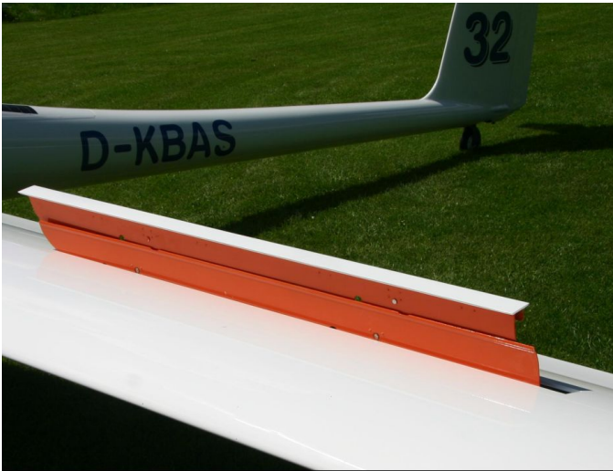
Fig. 6: Example for a tight airbrake (ASG 32): Both panels on the same side and only little cut-outs (Photo: Adolf Wilsch).
