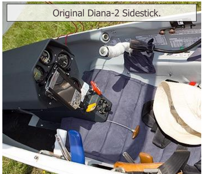
Sidestick with LX remote extends almost to the centre of the cockpit.
