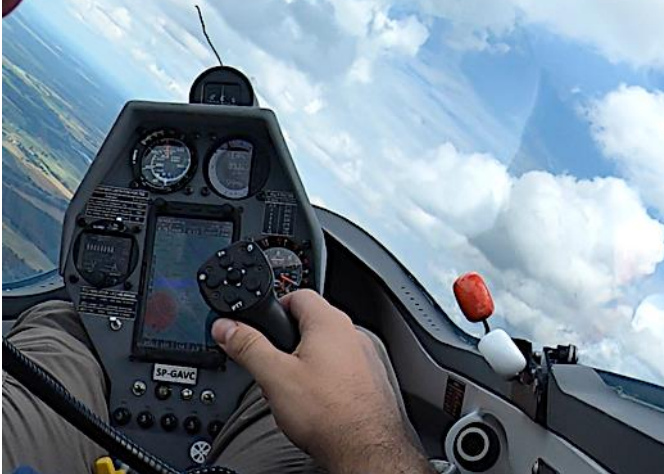
Sidestick with LX remote extends almost to the centre of the cockpit.
