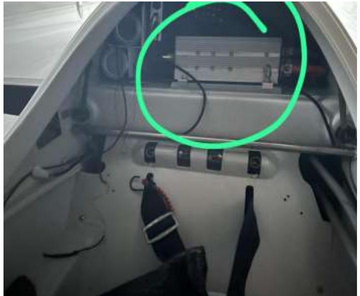
Figure 7: Position of FES Controller behind the head of GT
