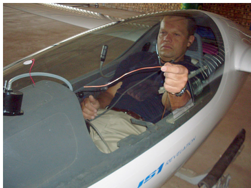
Figure 3. Measurement method for acoustic mapping of the boundary layer of the JS1.
