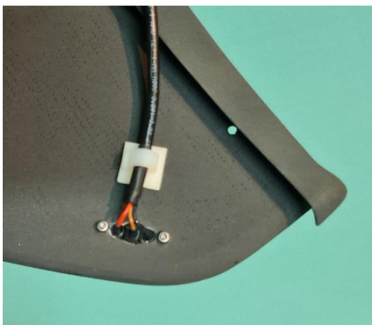
Put the counterpart cable through the panel. Use the plastic component (looks quite similar to the template) and tighten the screws (already used for the template).
