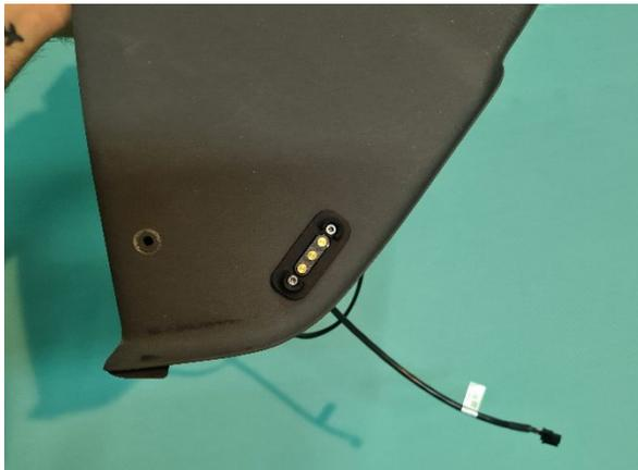
If the canopy-power interface and the counterpart are not aligned to each other, it is possible to make smaller adjustments on the canopy-power interface. Loosen the two screws and relocate the contact on the bracket. Larger deviations can only be solved by relocating the whole canopy-power interface on the canopy. (If this is unavoidable, please notice us via [info@sotecc.de](mailto:info@sotecc.de))
