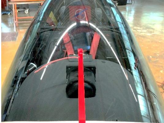
Define the middle of the canopy with a thin string or tape, then affix the template from outside. (Be careful: the small string may be positioned eccentrically!) Prior installing the canopy flash, clean the canopy with appropriate cleaning agent.
