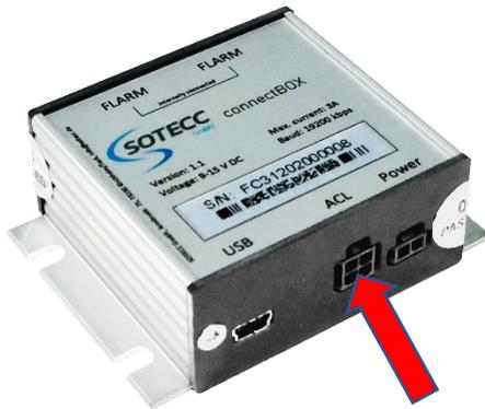
Plug the 4-pin connector cable of the counterpart (in the panel cover, see step 5, lower picture) into the ACL-port of the connectBOX.
