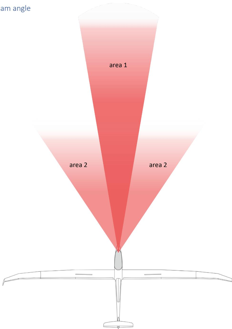
Area 1: ~ 18° concentrated light beam, which can be seen about 3500m, depending on the prevailing conditions.
