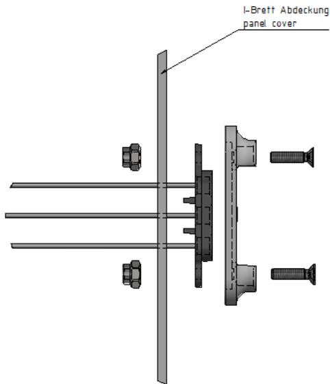
Fix the cable with the cable holder, install the suppressor, mount the panel cover and check if canopy-power interface and the counterpart align to each other by closing the canopy carefully.
