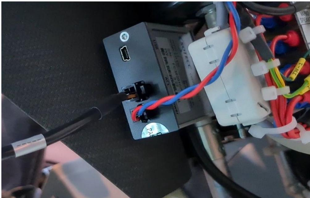
*Cable to the canopy-flasher at the top (ACL), connection to the on-board power supply at the bottom (Power). (The connectBOX is installed tilted 90 degrees to the right in the photo).*
