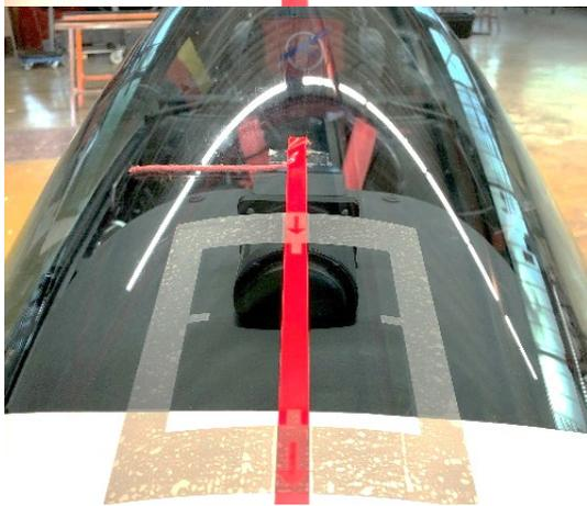
Then carefully remove the protective foil on the 3M adhesive strip with a cutter or something similar.
