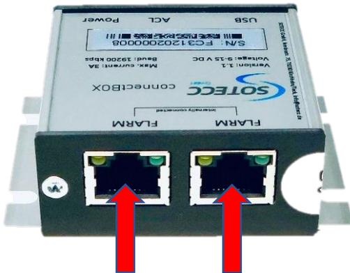
Finally connect FLARM® with RJ45 or RJ12 cable to the connectBOX.
