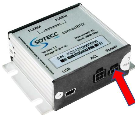
Connect the connectBOX to the on-board power supply with the 2-pin cable and install a 3-5 A fuse. If necessary shorten the power cable and then plug it into the power port of the connectBOX. To disconnect the connectBOX manually from the on-board power, place the switch between the power cable.
