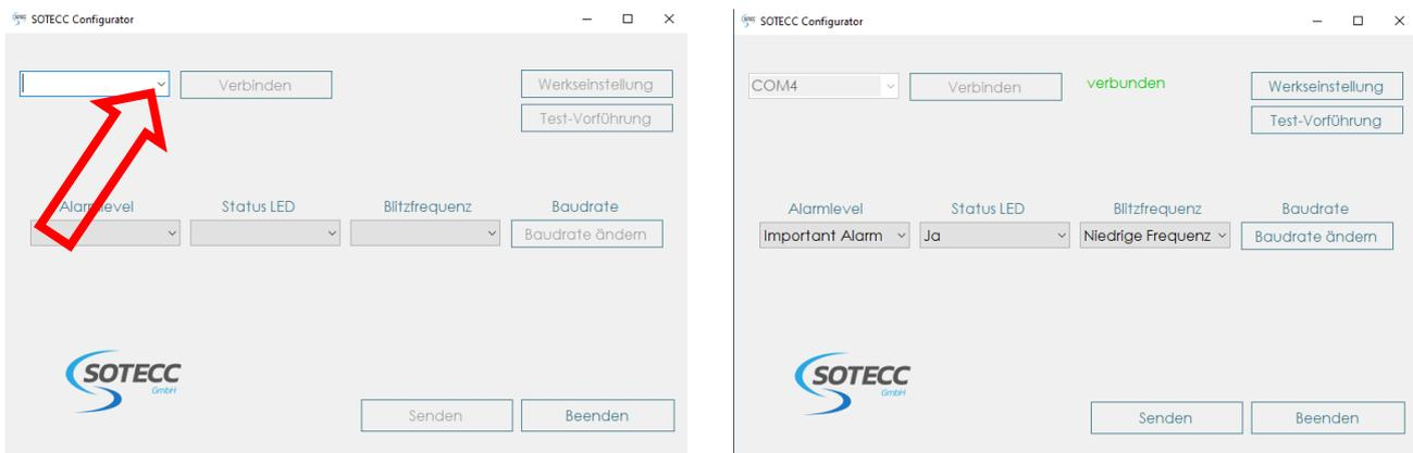
After successful connection, you will see the current (default) parameters and „connected“ in green next to the „connect“ button. If there is no response after 5 seconds, you may try to
