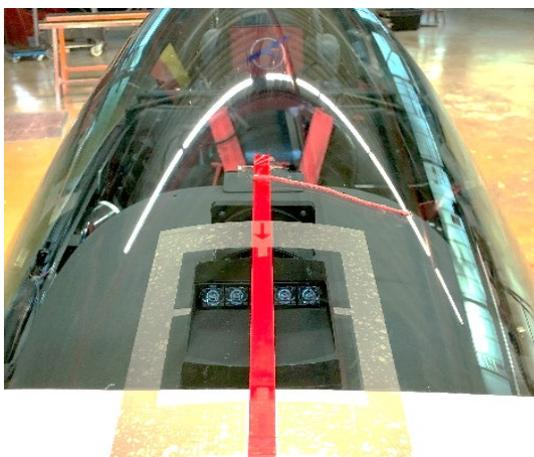
Subsequently align the canopy flash in accordance with the template, BUT press on the frontpart first, then swing the rear part up and press it on, this avoids air bubbles.
