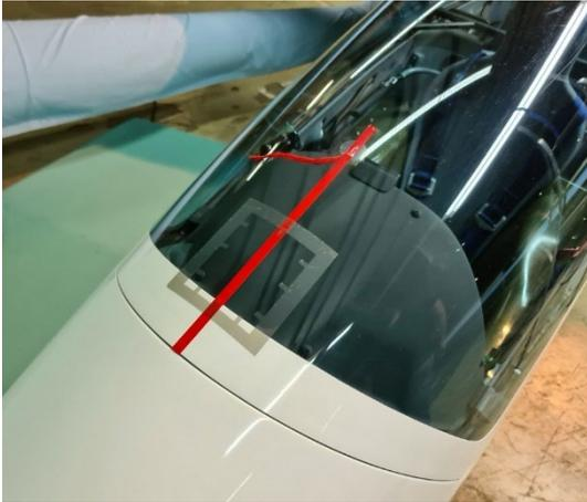
The front template spacers shall be positioned approx. 1mm behind the canopy paint edge. (direction to the tail). Various installation examples can be found [here](https://einbau.sotecc.de) (<https://einbau.sotecc.de>). The password can be found in the enclosed cover letter.
