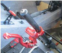
Allows to actuate the following calipers : 1x 1P27 EA-009/9.1 - 2x 2P27 calipers EA-006/6.2 - 1x 2P32 EA-002
