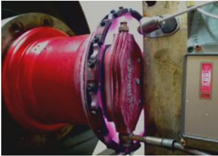
← *Braking test on our dynamometer to evaluate the kinetic energy capacity of the braking system caliper/disc*
