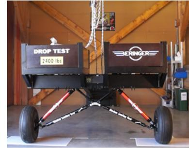
The patented ALG landing gear had to go through several tests for the certification process (FAA-EASA)
