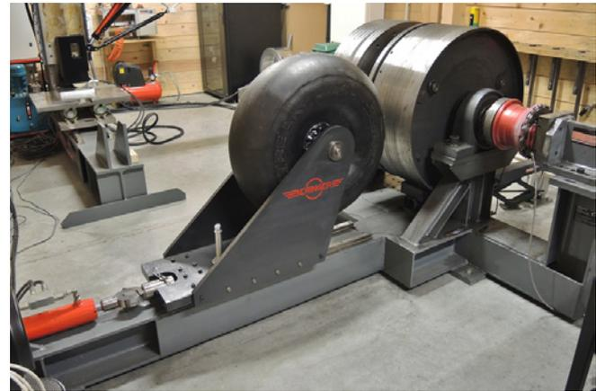
← ↑ 440,00Lbs Hydraulic press for ultimate load tests
