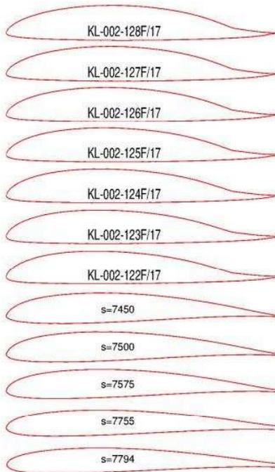
Fig. 10 Geometry of the wing and winglet airfoils.
