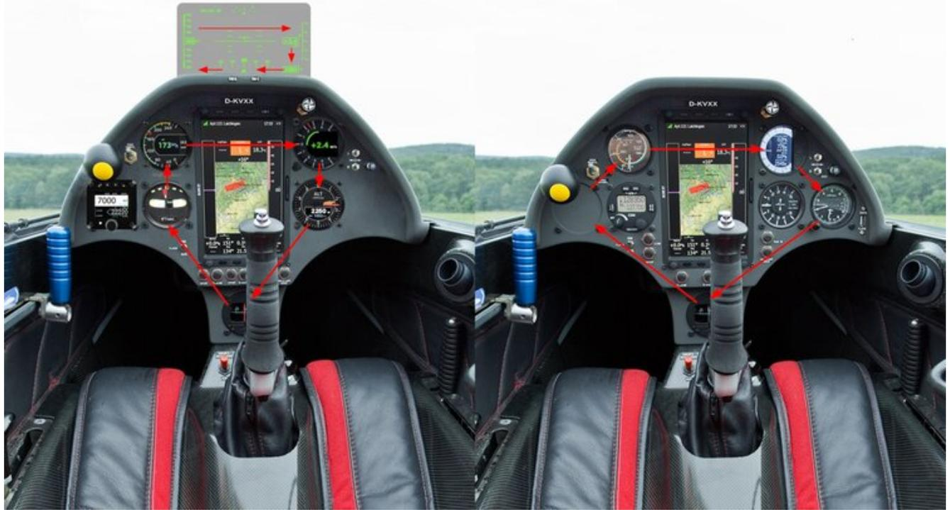
*Figure 5. Redesigned concept to the left and the reference plane to the right.*
