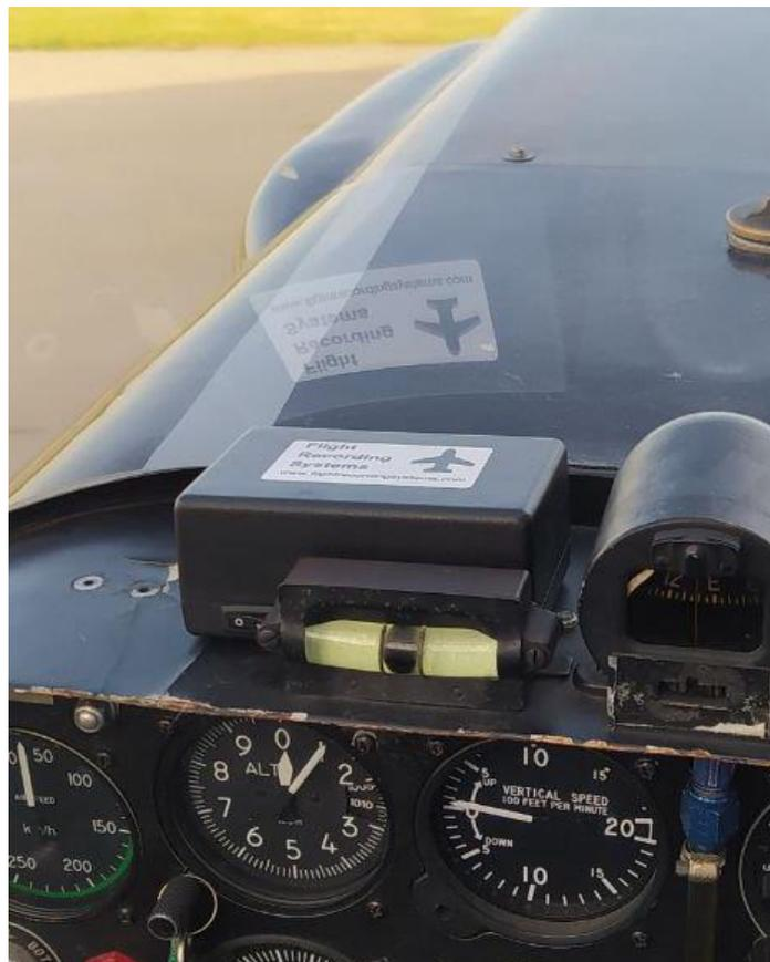
Figure 1 - Typical installation
