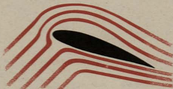
1. Wing close to stalling angle of attack
