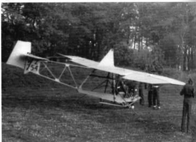
Grasshopper WZ754 suspended on its pendelbock at Bridlington School in 1976, with cadets. (P. J. V. Elliott, RAF Museum, Hendon, Ref PO19499)
